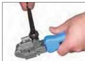
Step 2 Tighten the clamping nut
