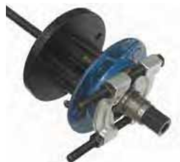
Inner Bearing Removal
