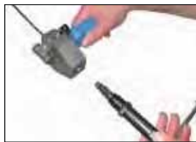
Step 3 Insert the punch and ram
