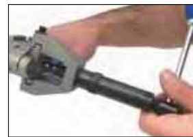
Step 4 Turn T-Bar to create the flare
